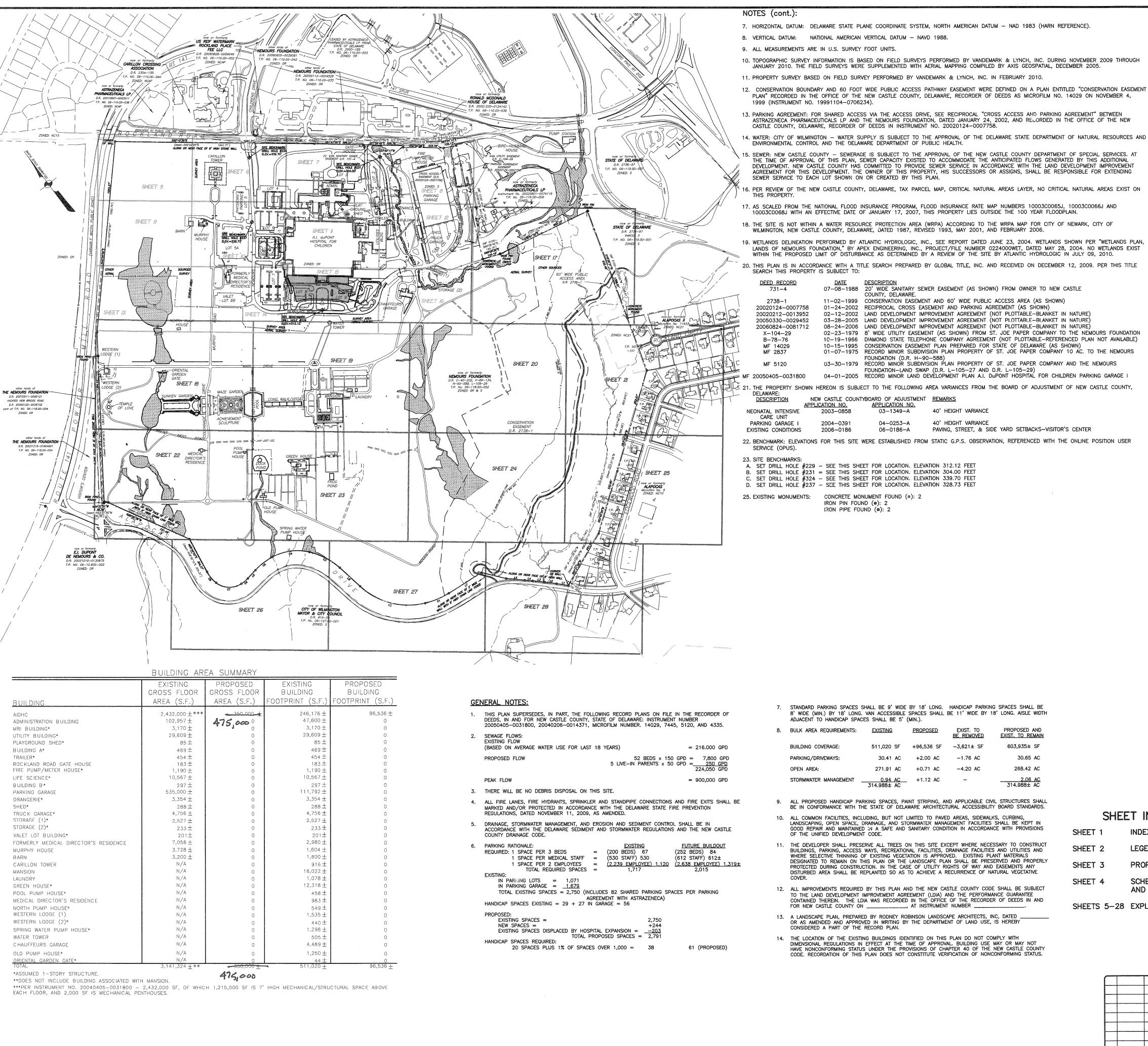
ADJACENT TO HANDICAP SPACES SHALL BE 5' (MIN.). 8. BULK AREA REQUIREMENTS: <u>EXISTING</u> PROPOSED BE REMOVED BUILDING COVERAGE: 511,020 SF +96,536 SF -3,621± SF PARKING/DRIVEWAYS -1.76 AC OPEN AREA: 271.91 AC +0.71 AC STORMWATER MANAGEMENT +1.12 AC
